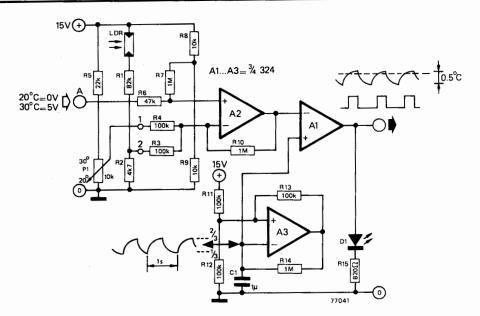
Although primarily designed to keep the water in an aquarium at a constant temperature, this circuit is also suitable for a number of other applications.
